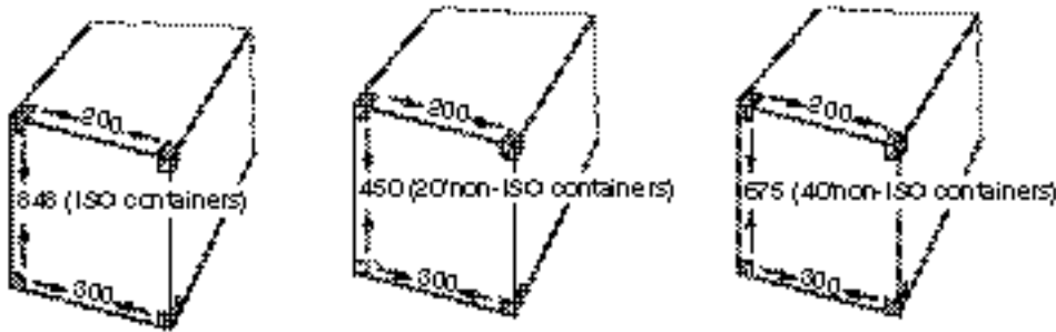
Figure 14 : Permissible transverse and vertical tensions on frames of 20' and 40' containers
